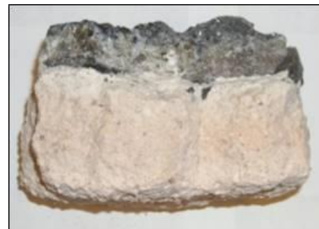
Slag and metal infiltration of conventional silica-based dry-vibratable
