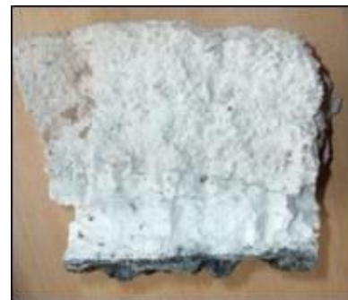
Slag and metal infiltration of LGS silica
