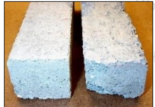
TUFFLOOR Standard Concrete Thermal Cycling to 1400°F (760°C)
