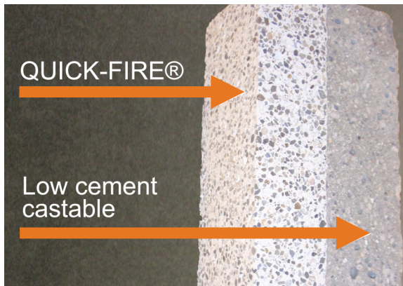
QUICK-FIRE® bonding to existing refractory
