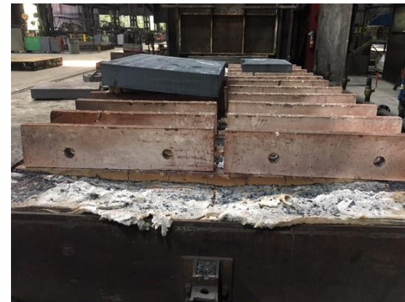
The same ARMORMAX® 70 SR pier blocks after 3.5 years of continuous service
