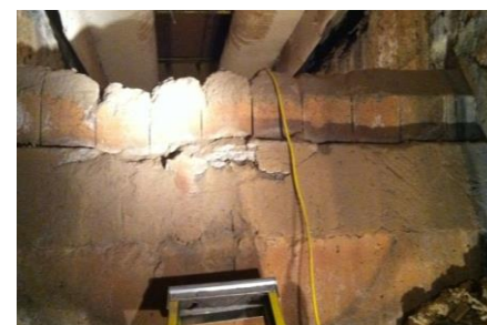
METAL-ROK® cricket wall shapes after 15-month campaign. Steel support structure compromised.
